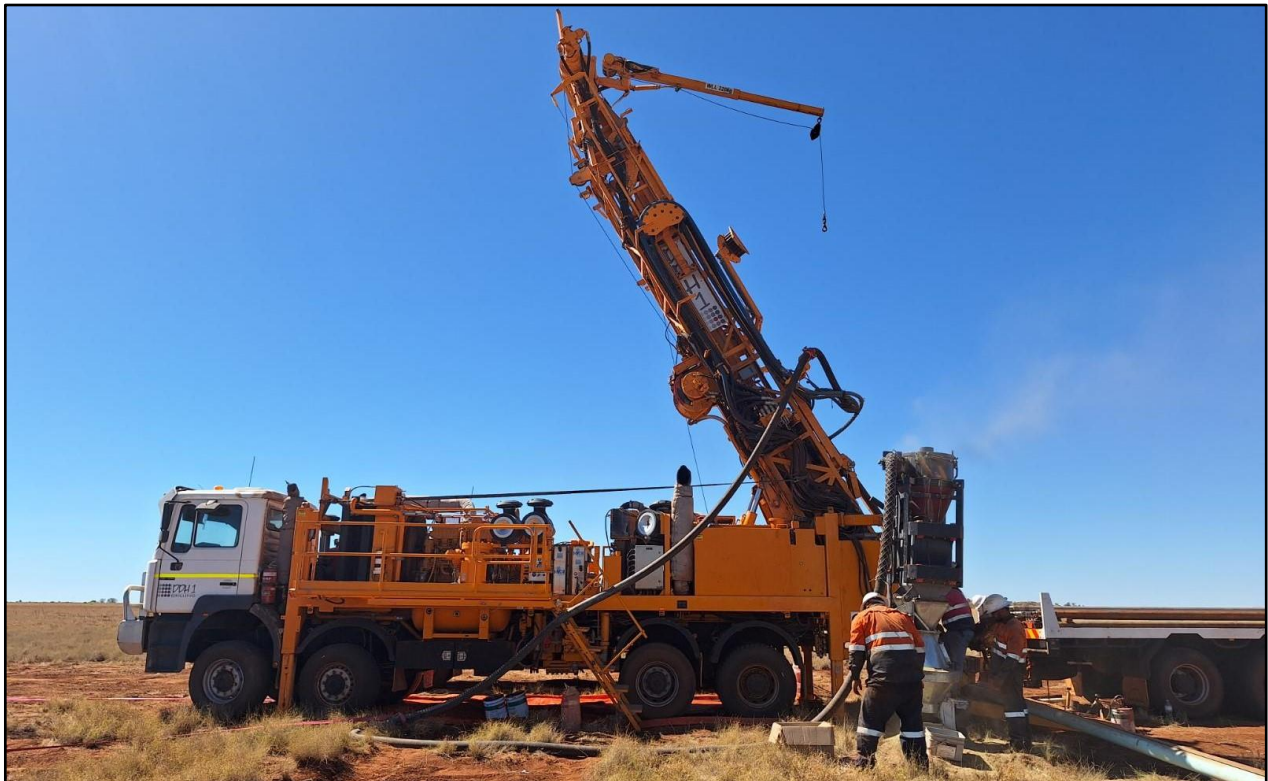
Image 1: DDH1 multi-purpose drilling rig pre-collaring SBDD006 testing the new EM conductor
