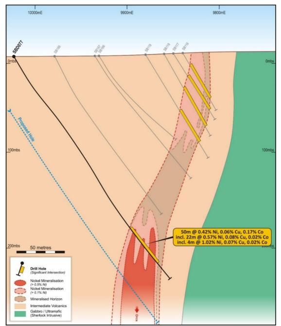
Figure 4 - Sherlock Bay cross section 19,600mE, Discovery deposit with high-grade Ni sulphide target
