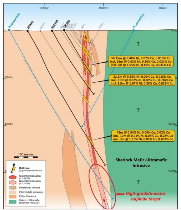
Figure 3: Symonds Nickel Deposit, Cross Section 20,760mE showing high-grade nickel sulphide target
