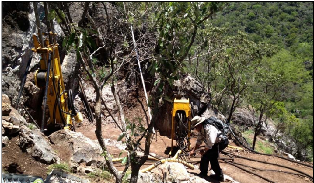
Figure 3 – At Pad 5, a Company geologist examines outcropping copper mineralisation adjacent to the new contractor's man-portable diamond drill rig.
