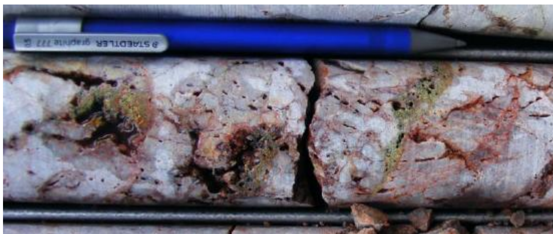
Figure 4 - Mineralised rocks from drilling at Kaskara in drillhole KSK021. Gossanous zones (red-brown, top image) appear to be sporadically mineralised and can be correlated between surface and drill hole. Mottramite (yellow-green to black, bottom image) commonly occurs as clots and vein infills in the highly oxidised and brecciated rocks.
