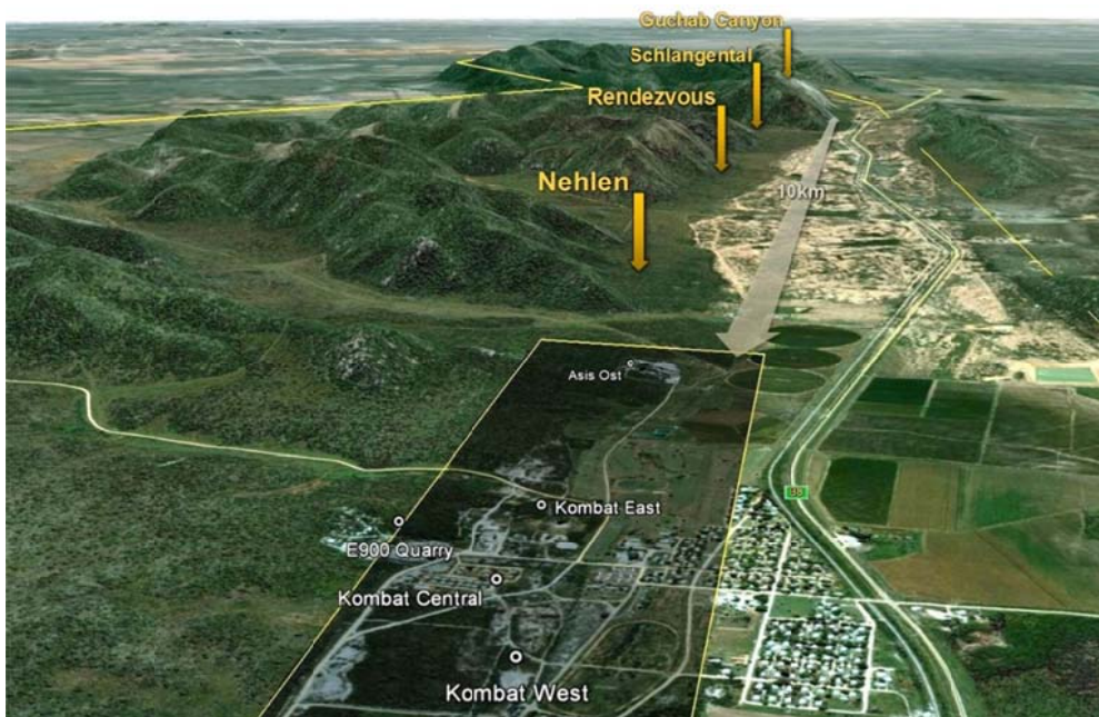
Figure 3 – Oblique view east from the Kombat copper mine (foreground, excised area shaded) along strike to Sabre's series of copper targets (yellow) at Nehlen, Rendezvous, Schlangental & Guchab Canyon in the Kombat East Target Area. The licence boundary is shown in yellow.
